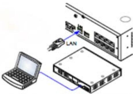
2. Connect the installation laptop via an R45 lead to the LAN socket on the control unit rear panel.
